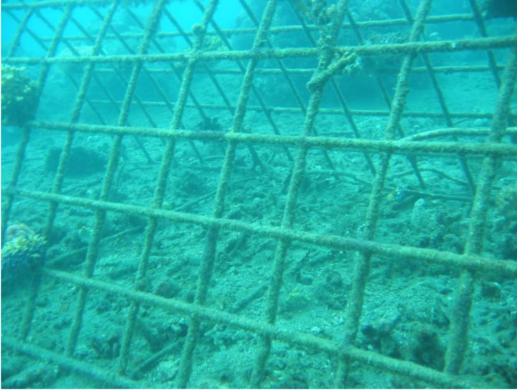
Figure 1: Algae covered on biorock, 1-2mm, under there is a thin layer (less than 1mm) of calcium deposition.
